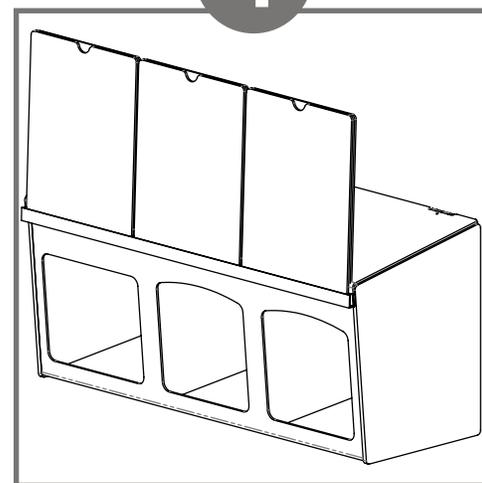
Slide up to two additional sign holders into groove, each butting up against the previous holder.
