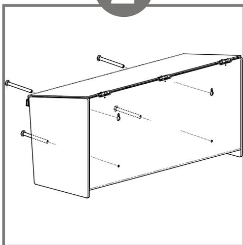
Dispenser should be mounted securely to a wall through keyholes and through-holes in back with screws approved by building maintenance.
