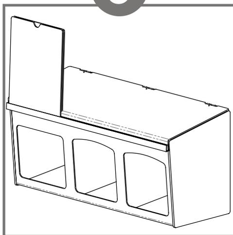
Optional sign holders, MP-035, are attached by sliding into groove on front edge of dispenser lid.
