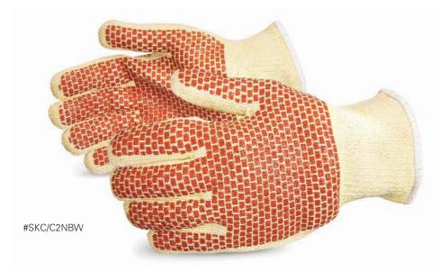
Nitrile applied to hot mill gloves makes a huge improvement over PVC because it withstands higher temperatures, and unlike PVC, will not melt or mar surfaces or leave smears on objects behind the way PVC will. We use a unique process to apply nitrile blocks across the palms so that grip stays solid for the life of the glove, rather than peeling off with repeated use and laundering.
