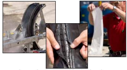
During testing for CE certification in July 2009, TurtleSkin MFA WaterArmor allowed zero penetration at 40,000psi with a swipe speed of 1.6 feet/second.
